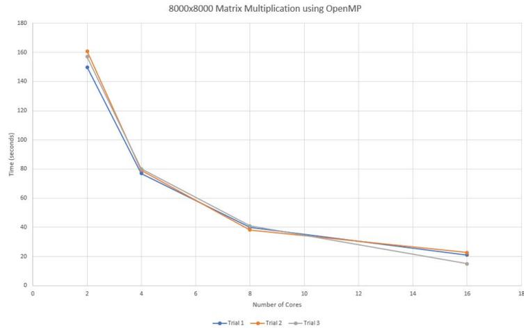
The Comet supercomputer runs tasks on multiple threads, which allows them to be completed more efficiently by splitting the load between the threads. We compared the difference between two multithreading APIs to run an example computation task. We noticed that MPI completed the example task faster than OpenMP, but the gap started to close at higher core numbers as MPI produced more diminishing returns.
